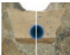
Traditional pipelaying in trenches and adapted for pipes made of PE100 RC.
